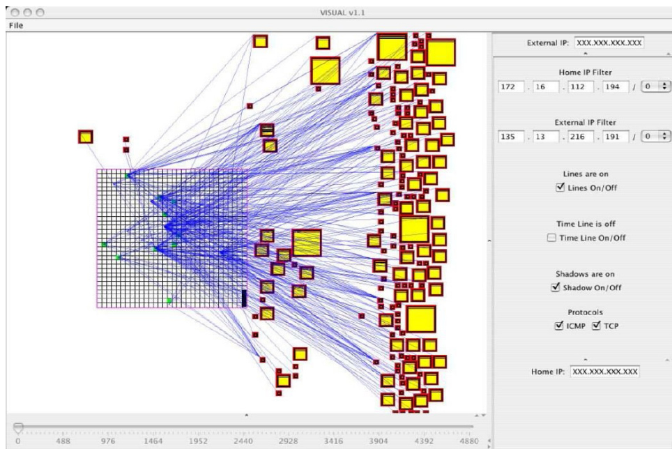
Figure 3-3: VISAUL displaying 80 hours of network data with 915 communication between a home network of 1020 hosts and 183 external hosts [Ball 2004: 58]
