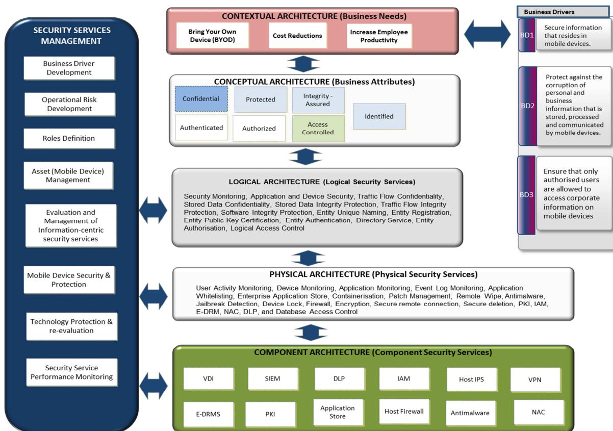
**Figure 3-1: Utopian Reference Architecture Framework Based on SABSA**
