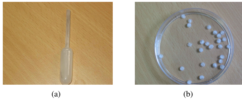
Figure 4.10: (a) Plastic pipette filled with wax and (b) sliced sections of the pipette
