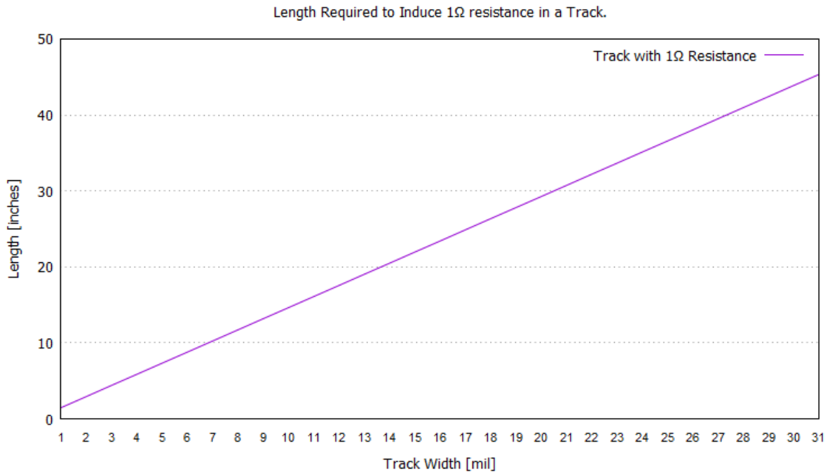
Figure 5.10: Trace Dimensions Contributing a Net Resistance of 1 Ohm
